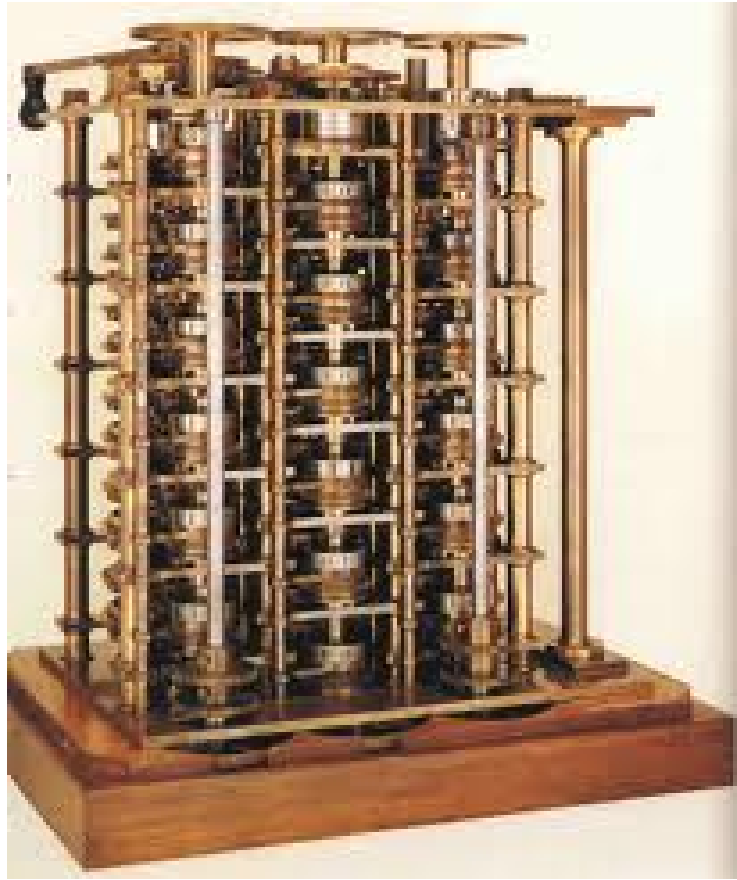
Figure 5: Charles Babbage's difference engine, the forerunner of modern computers.
