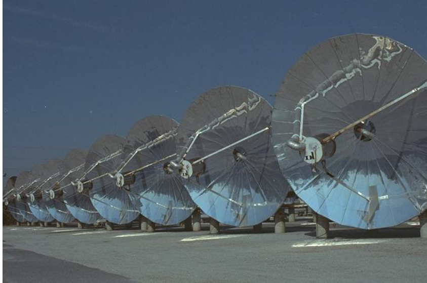
Figure 1: A row of 7 meter diameter stamped sheet metal solar concentrators in Georgia USA. The metal is covered with special high-reflection foil.
