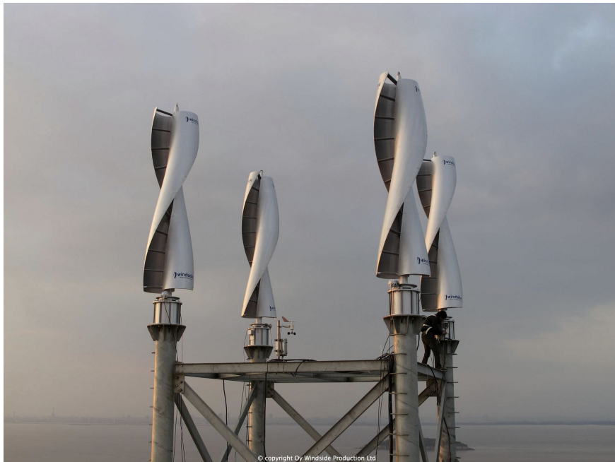
Figure 2.6: Vertical axis wind turbines.
