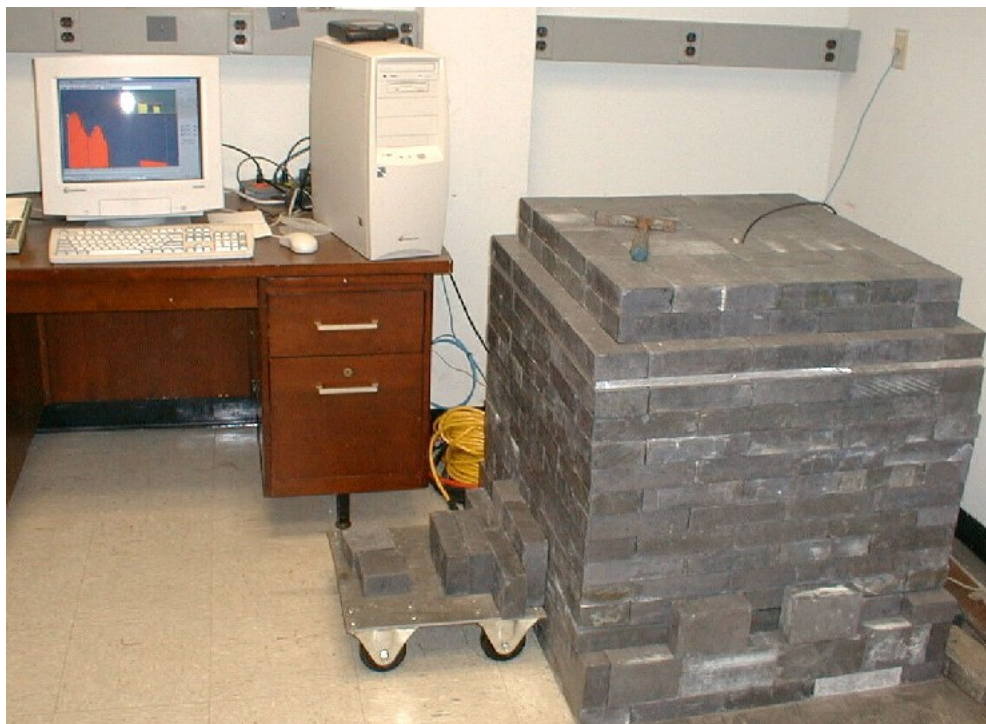
Fig. 2: ^{152}\text{Eu} is used as a reference source for calibrating gamma-ray spectrometer systems like the one pictured here. (Photo Source: Snyder and Duval, 2003. U.S. Geological Survey Open-File Report 03-029) [455].
