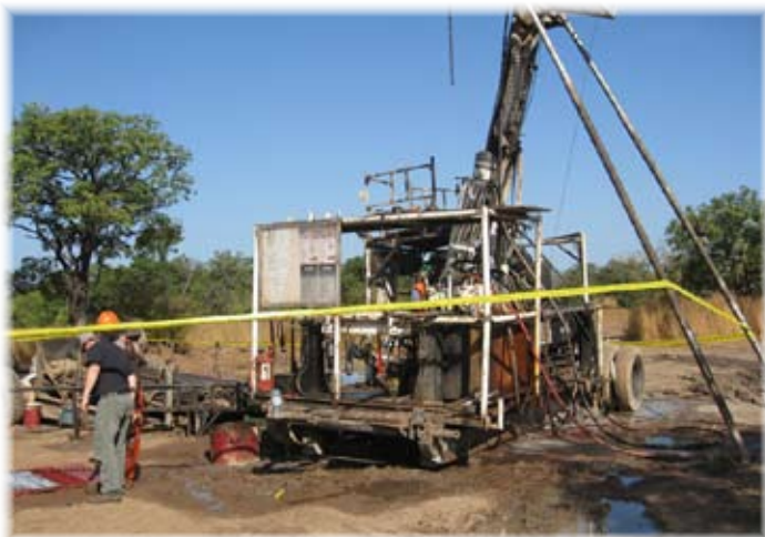
Drilling machine for core drilling in Falea Photo Rockgate
