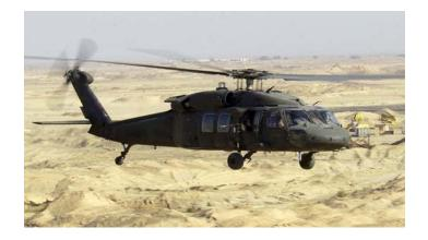
**Description:** The BLACKHAWK is a twin engine, single-rotor helicopter that is designed to carry a crew of four and a combat equipped squad of eleven or an equal cargo load. It is also capable of carrying external loads of up to 6,000 lbs. The prime contractor is Sikorsky Aircraft of Stratford, CT.
