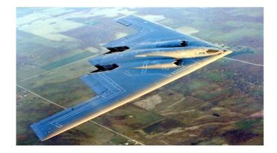
**Description:** The B-2 is an intercontinental bomber that employs low observable technology to achieve its mission. The bomber is an all-wing, two-place aircraft with twin weapon bays. Four General Electric F-118-GE100 aircraft engines power the B-2. Northrop-Grumman Corporation, El Segundo, CA is the prime contractor for the B-2s.
