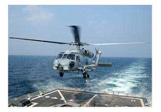
**Description:** The MH-60R Multi-Mission Helicopter Upgrade program provides battle group protection and adds significant capability in coastal littorals and regional conflicts. The upgrade scope includes new H-60 Series airframes, significant avionics improvements, and enhancements to the acoustic suite, new radars and an improved electronics surveillance system. Prime contractors are Sikorsky Aircraft of Stratford, CN for the airframe and Lockheed Martin of Owego, NY for the avionics.
