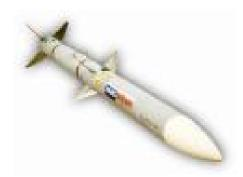
**Description:** The Advanced Medium Range Air-to-Air Missile (AMRAAM) is an all-weather, all-environment radar guided missile developed to improve capabilities against very low-altitude and high-altitude, high-speed targets in an electronic countermeasures environment. AMRAAM is a joint Navy/Air Force program led by the Air Force. The prime contractor is Raytheon Corporation, Tucson, AZ.
