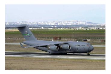
**Description:** The C-17 is a wide-body aircraft capable of airlifting outsized and oversized payloads over intercontinental ranges, with or without in-flight refueling. Its capabilities include rapid direct delivery of forces by airland or airdrop into austere tactical environments and is capable of performing both intertheater and intratheater airlift missions. The major contractors are Boeing, Long Beach, CA (Airframe) and Pratt-Whitney, East Hartford, CT (Engine).
