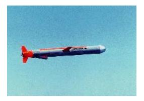
**Description:** The Tactical Tomahawk is a Navy cruise missile weapon system is a long-range conventional warhead system which is sized to fit torpedo tubes and capable of being deployed from a variety of surface ship and submarine platforms. The prime contractor is Raytheon, Tucson, AZ.
