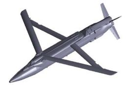
**Description:** The Small Diameter Bomb (SDB) is a joint Air Force and Navy program led by the Air Force to provide a conventional small sized, precision guided, standoff air-to-ground weapon that can be delivered from both fighters and bombers. Boeing Corporation of St. Charles, MO is the prime contractor.
