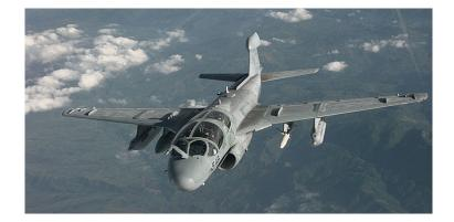
**Description:** The EA-6B Prowler is a 4-seat twin engine derivative of the A-6 Attack aircraft that is equipped with a computer-controlled electronic surveillance and control system and high power jamming transmitters. The overall goals of the modification program are to upgrade the airframe structure and avionics systems to increase the life of the aircraft and to expand the aircraft's jamming capabilities. The prime contractor is Northrop Grumman Corporation, Bethpage, NY.
