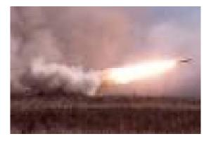
**Description:** The High Mobility Artillery Rocket System (HIMARS) consists of a C-130 transportable, wheeled, indirect fire, rocket/missile system capable of firing all rockets and missiles in the current and future Multiple Launch Rocket System (MLRS) family of munitions. The prime contractor is Lockheed Martin Missiles and Fire Control, Dallas, TX.
