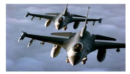
**Description:** The F-16 is a single seat, fixed wing, high performance fighter aircraft powered by a single engine. The advanced technology features include a blended wing body, reduced static margin, and fly-by-wire flight control system. Prime contractors are Lockheed-Martin of Fort Worth, TX for the airframe and Pratt and Whitney of East Hartford, CT and General Electric, Evendale, OH for the engine.
