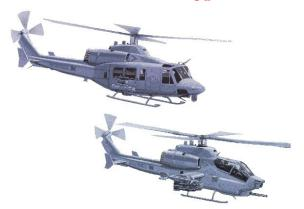
**Description:** The H-1 Helicopter Upgrades program converts AH-1W and UH-1N helicopters to the AH-1Z and UH-1Y, respectively. The upgraded helicopters will have increased maneuverability, speed, and payload capability. The upgrade scope includes a new four-bladed rotor system, new transmissions, a new four-bladed tail rotor and drive system, and upgraded landing gear. The prime contractor is Bell Helicopter Division, Fort Worth, TX.
