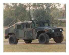
**Description:** The High Mobility Multi-purpose Wheeled Vehicle (HMMWV) is a light, highly mobile, diesel powered, air transportable and air droppable, 4-wheel drive tactical vehicle. The HMMWV can be configured through the use of common components and kits to become a cargo/troop carrier, armament carrier, shelter carrier, ambulance, and TOW and Stinger weapons carrier. The prime contractor is AM General of Mishawaka, IN.
