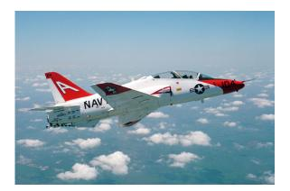
**Description:** The T-45S GOSHAWK is a derivative of the British Aerospace HAWK aircraft. The T-45 Training System will integrate aircraft, simulators, academics, and a training management system into a replacement for current intermediate and advanced phase training aircraft. The prime contractor is Boeing Aircraft Company, St. Louis, MO; British Aerospace of Kingston, England provides the center and aft fuselage; and Rolls Royce, Ltd of Bristol, England provides the engine.
