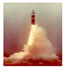
**Description:** The TRIDENT II (D-5) is a submarine launched ballistic missile with greater range, payload capability and accuracy than the TRIDENT I. The major contractor is Lockheed Martin Missiles and Space Company, Sunnyvale, CA.
