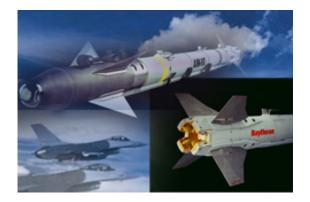
**Description:** The AIM-9X short range air-to-air missile provides a launch and leave, air combat missile that uses passive infrared energy for acquisition and tracking of enemy aircraft. AIM-9X is a joint Navy/Air Force program led by the Navy. The prime contractor is Raytheon Corporation, Tucson, AZ.
