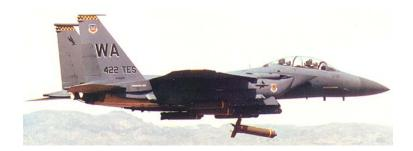
**Description:** The Wind Corrected Munitions Dispenser (WCMD) guidance kit for the Combined Effects Munition, Gator Mine, and Sensor Fuzed Weapon provides inertial navigation to correct for the effects of wind transients and ballistic errors caused by wind when these munitions are released from medium to high altitudes. The contractor is Lockheed-Martin, Orlando, Florida.
