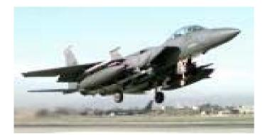
**Description:** The F-15E is a twin-engine, two man crew, fixed swept wing aircraft. The F-15E maintains the basic F-15 air superiority characteristics while adding air-to-surface weapons capability. Prime contractors are Boeing of St. Louis, MO for the airframe, and Pratt and Whitney of East Hartford, CT for the engine.
