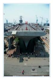
**Description:** The CVN Refueling Complex Overhaul program is a program to refuel and upgrade Nimitz class aircraft carriers at about their mid-life of 25 years. The refueling and upgrades will provide for reliable operations during the remaining ship life using only the normal maintenance cycle. The contractor is Northrop-Grumman, Newport News, VA.
